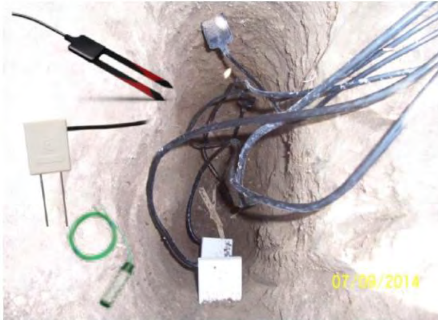
Figure 2. Three different soil moisture sensors (Watermark, CS655, and Decagon 10HS) installed at different depths (1, 2, and 3 feet) at the SWREC plot and a farmer's field.
